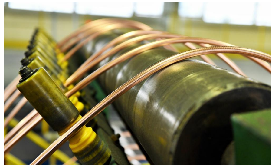
Figure 12. Copper wire drawing process; source: KGHM Polska Miedź
