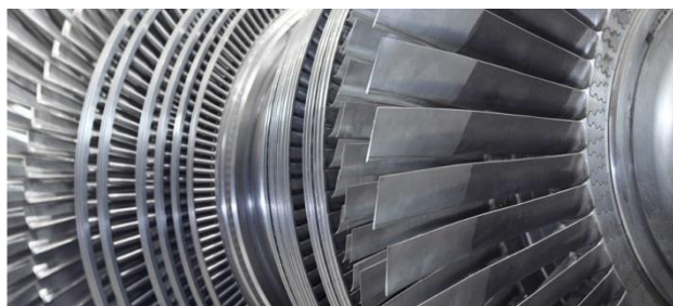
Nickel-containing superalloys are used in turbine blades of jet engines (AMG Superalloys)
